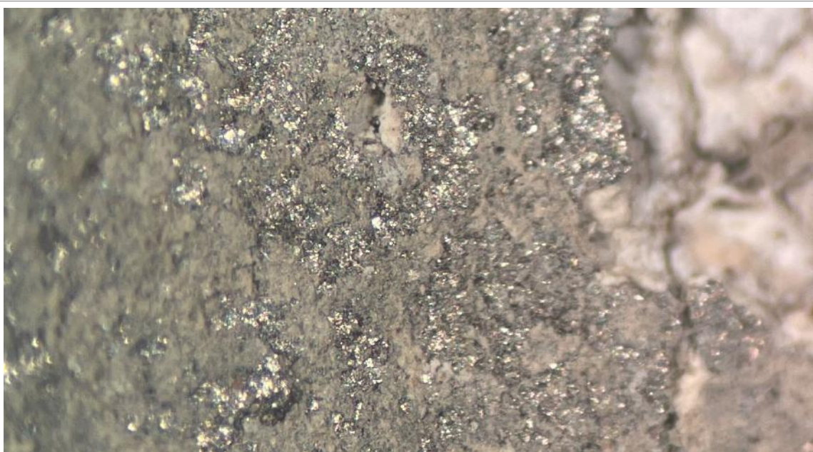
Figure 16: “Horse” Sculpture, Microscopic Image of Hand Sample of Coating Sample 1 Metallic gray layer exposed in hand sample, which could potentially be an aluminum paint, used as a protective layer beneath the final white presentation layer.
