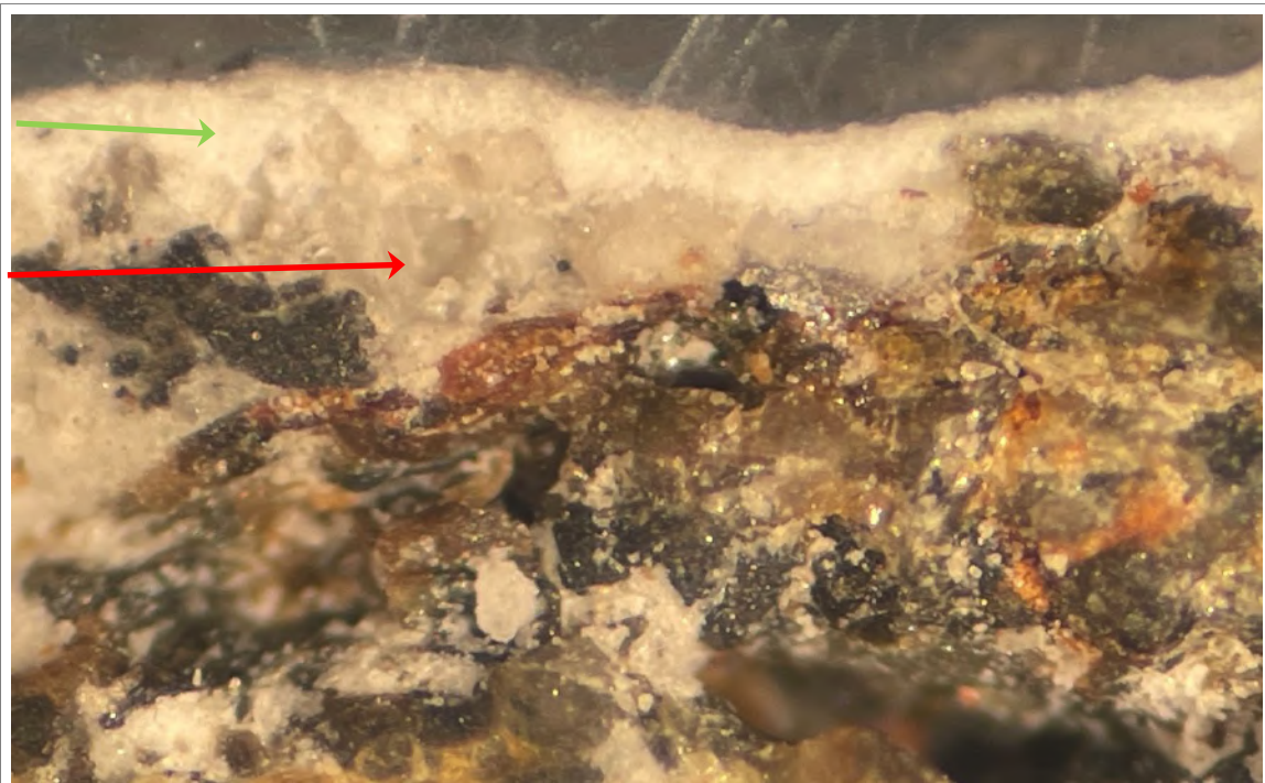
Figure 10: “Hemlock Tree,” Underside of Tree Location, Microscopic Image of Coating Sample 3 in Cross Section Earliest extant layer appears to be a white cementitious skim coating (indicated in red), followed by a thin white layer (indicated in green), possibly a thin paint or laitance from the skim coating.
